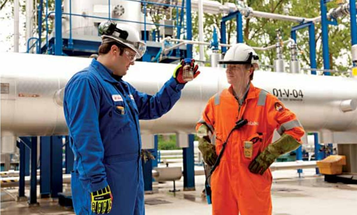
Michael Olson (left), ExxonMobil Upstream Research, and René Ubachs, ProLabNL, examine a water sample from the subsea separator qualification trials in the Netherlands. ExxonMobil and ProLabNL jointly developed safe work practices for the high-pressure tests, including sampling procedures and personal-protective equipment requirements.
