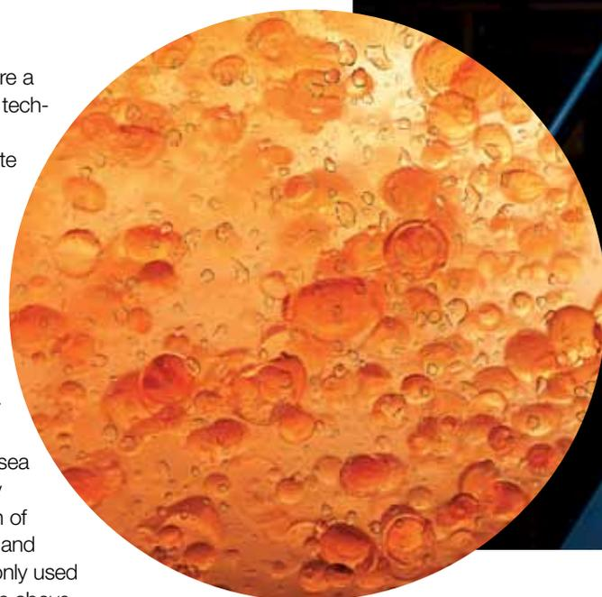
Adam Bymaster (left) and Ed Grave, ExxonMobil Upstream Research, observe low-pressure testing of a pipe separator to be employed in the company's innovative subsea compact separation system. Low-pressure, transparent testing with model fluids provides insight into complex fluid behavior, such as droplet coalescence and the breakdown of foams and emulsions shown in the inset.
